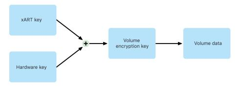
If FileVault is turned on later — a process that is immediate because the data has already been encrypted — an anti-replay mechanism helps prevent the old key (based on hardware UID only) from being used to decrypt the volume. The volume is then protected by a combination of the user password with the hardware UID as previously described.
