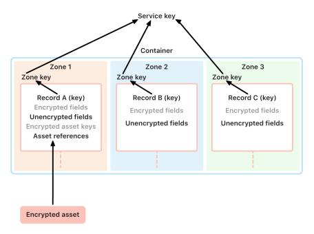
The security of encrypted data in CloudKit relies on the security of the corresponding encryption keys. CloudKit service keys are divided into two categories: end-to-end encrypted and available-after-authentication.
