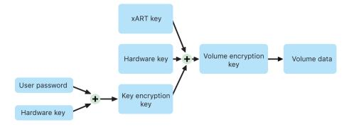
On a Mac with Apple silicon and those with the T2 chip, all FileVault key handling occurs in the Secure Enclave; encryption keys are never directly exposed to the Intel CPU. All APFS volumes are created with a volume encryption key by default. Volume and metadata contents are encrypted with this volume encryption key, which is wrapped with a key encryption key (KEK). The KEK is protected by a combination of the user's password and hardware UID when FileVault is turned on.
