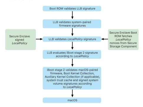
The chip executes code from the Boot ROM in the first step in the chain of trust. macOS secure boot on a Mac with Apple silicon verifies not only the operating system code itself, but also the security policies and even kexts (supported, though not recommended) configured by authorised users.
