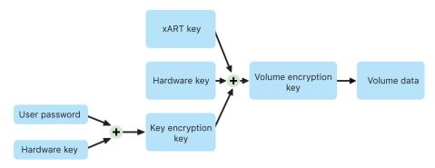
On a Mac with Apple silicon and those with the T2 chip, all FileVault key handling occurs in the Secure Enclave; encryption keys are never directly exposed to the Intel CPU. All APFS volumes are created with a volume encryption key by default. Volume and metadata contents are encrypted with this volume encryption key, which is wrapped with the class key. The class key is protected by a combination of the user's password and the hardware UID when FileVault is turned on.
