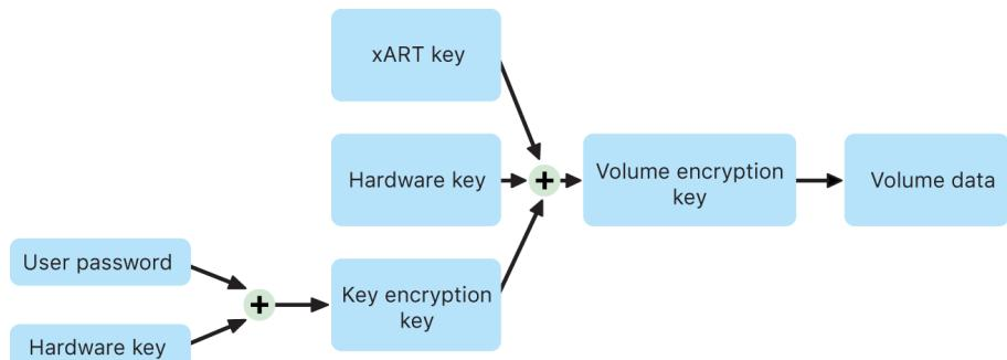
On a Mac with Apple silicon and those with the T2 chip, all FileVault key handling occurs in the Secure Enclave; encryption keys are never directly exposed to the Intel CPU. All APFS volumes are created with a volume encryption key by default. Volume and metadata contents are encrypted with this volume encryption key, which is wrapped with a key encryption key (KEK). The KEK is protected by a combination of the user's password and hardware UID when FileVault is turned on.
