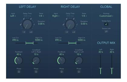
The parameters for the left and right delays are identical. The following descriptions apply to both channels. Global and Output Mix parameters are described after the channel parameters.
