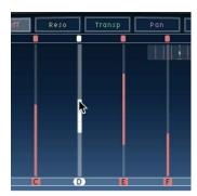
When the highpass filter cutoff frequency value is lower than that of the lowpass cutoff frequency, only one line is shown. This line represents the frequency band that passes through the filters—in other words, the filters act as a bandpass filter. In this configuration, the two filters operate in series which means the tap passes through one filter first, then the other.
