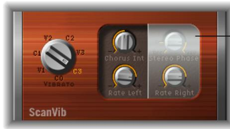
The stereo parameters of the mono version of the Scanner Vibrato are hidden behind a transparent cover.
