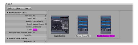
The order of the icons from left to right defines the order in which tracks and parameters are arranged and displayed on the devices.
